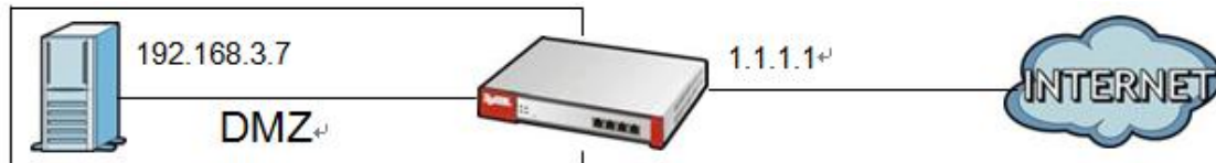
Figure 45 Public Server Example Network Topology
