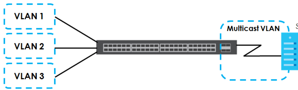
Figure 144 MVR Network Example
