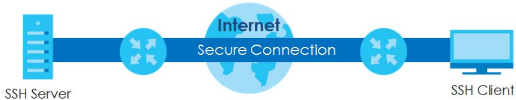
Figure 261 SSH Communication Example
