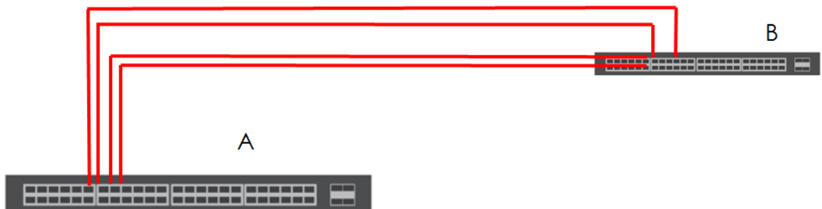
Figure 125 Trunking Example - Physical Connections
