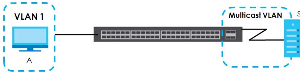
Figure 145 MVR Multicast Television Example
