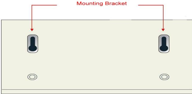
Figure 2-1 Wall-Mounting Bracket - Bottom of Wireless Subscriber Gateway
