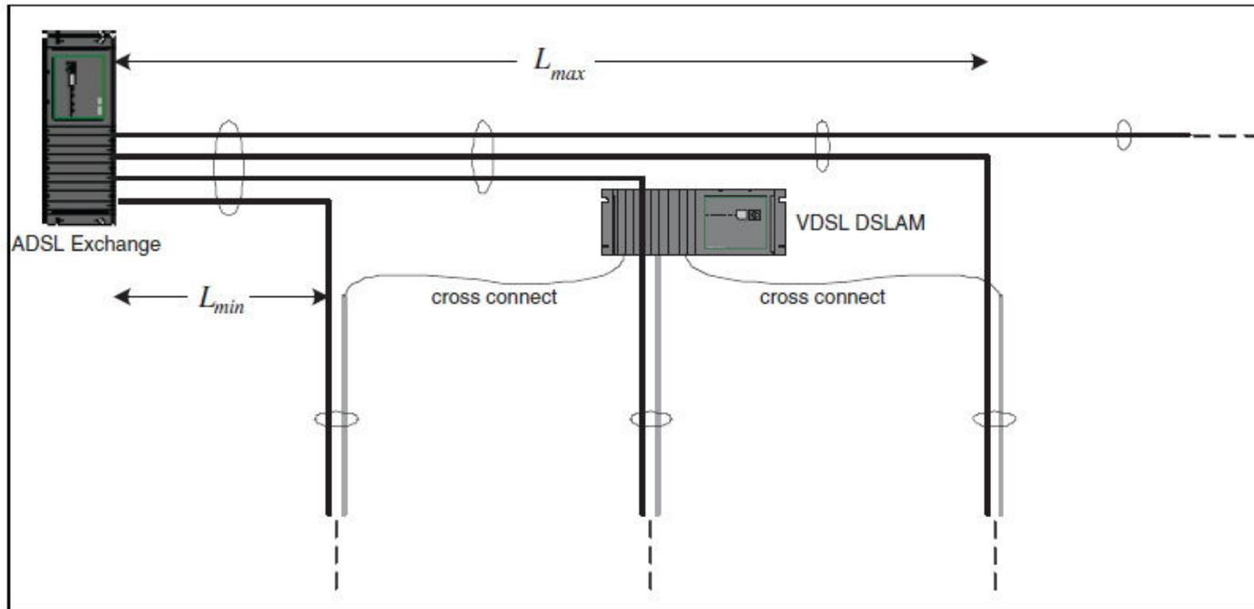
**Figure 5.6.3 DPBO Scenario with Cross-connections**
