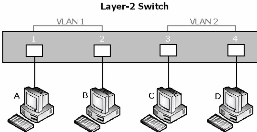
**IEEE 802.1Q (tag) -based VLANs** enable the Ethernet functionality to propagate tagged packets across the bridges and provides a uniform way for creating VLAN within a network then span across the network. For egress packet, you can choose to tag it or not with the associated VLAN ID of this port. For ingress packet, you can forward this packet to a specific port as long as it is also in the same VLAN group.
