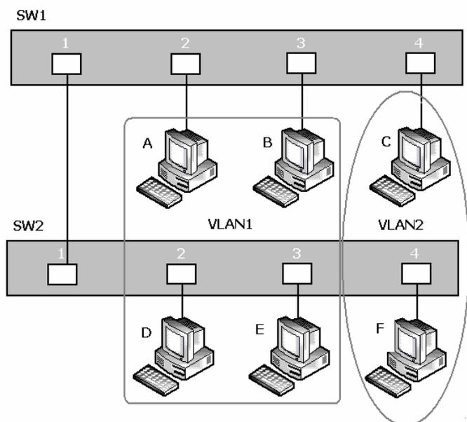
The NV-1602S supports both port-based VLAN and tag-based (802.1Q) VLAN modes. The default configuration is tag-based (802.1Q) VLAN. In the 802.1Q VLAN, initially, all ports on the switch belong to default VLAN, VID is 1.
