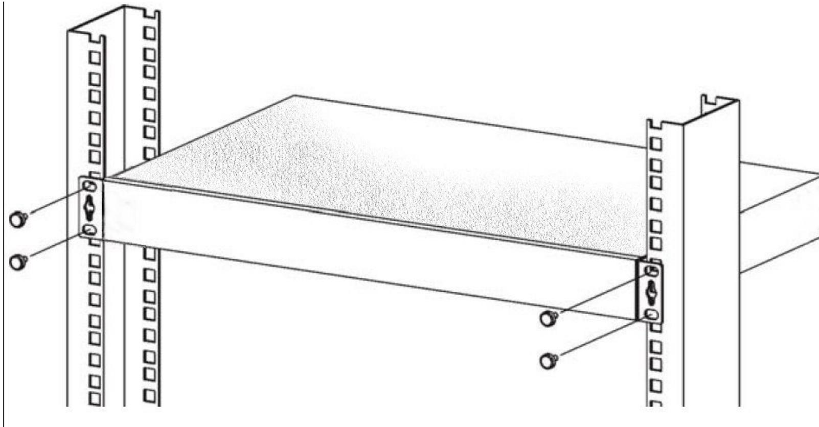
2. Using a screwdriver, install the M5 flat head screws through the mounting bracket holes into the rack.
