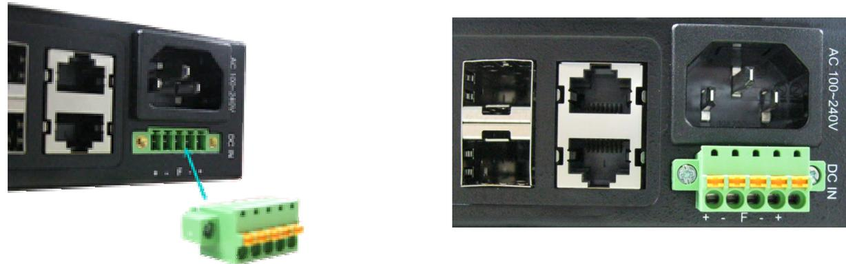
The NV-1602S can be powered two -48V DC power supply. The DC power interface is a 5-pin terminal block is located below the AC socket of the DSLAM. 2P is for accommodating one DC power input and other 2P is for accommodating another DC power input. The center pin of the terminal block is FGND. The DC power should be connected to a well-fused power supply. When using a DC voltmeter, Please check for proper voltage: -75V ~ -36 VCD, and make sure that the polarity is correct.
