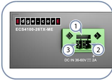
**i** **Note:** Before wiring the DC plug or connecting power to the switch, ensure that power to the feed lines is turned off at the supply circuit breaker or disconnected from the power bus.
