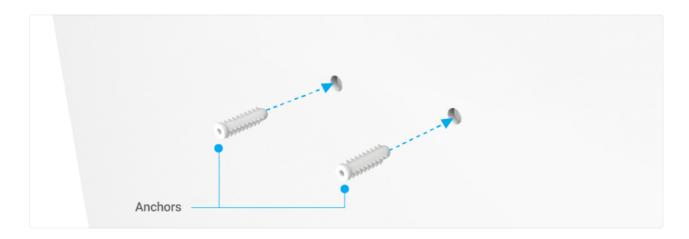
4. Insert and tighten the **Screws** into the **Anchors**, but leave the screw head sticking out so you can hang the **Controller** on it.
