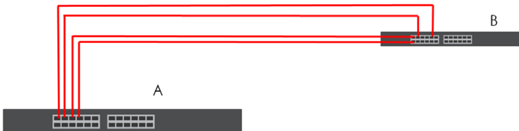
Figure 131 Trunking Example – Physical Connections
