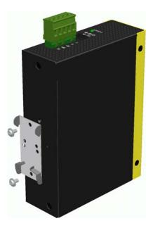
2. Attach bracket to the lower edge of the DIN rail and push the unit upward a little bit until the bracket can clamp on the upper edge of the DIN rail.
