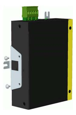
3. Screw the switch unit on a panel and the locations for screws are shown below:
