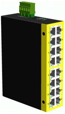
The switch provides sixteen 10/100Mbps copper ports for connections to Ethernet and Fast Ethernet devices. With the featured auto-negotiation function, the switch can detect and configure the connection speed and duplex automatically. The switch also provides auto MDI/MDI-X function, which can detect the connected cable and switch the transmission wire pair and receiving pair automatically. This auto-crossover function can simplify the type of network cables used.
