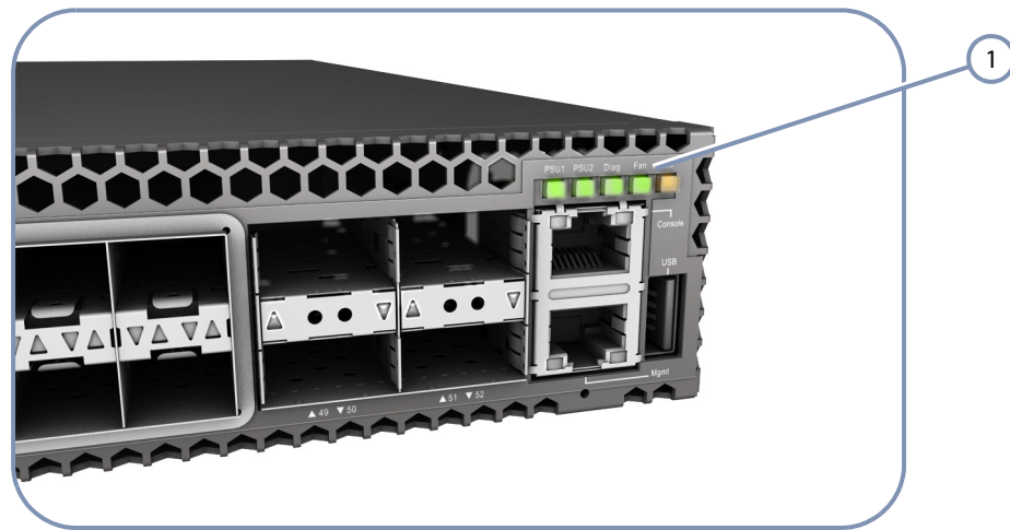
1 System Status LEDs.
