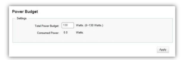
Total Power Budget: Enter the amount of power the Switch can provide to all ports.
