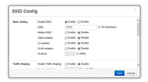
Enable SSID: Select to enable or disable the SSID broadcasting.
