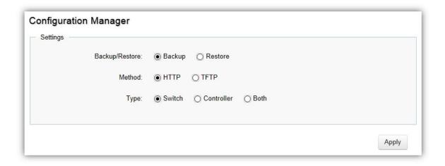
Click Apply to download configuration settings to your computer or a TFTP server, or to upload previously saved configuration file to the system.
