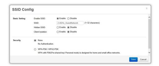
Enable SSID: Select to enable or disable the SSID broadcasting.
