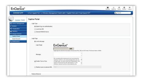
Login Type: Defines the mechanism by which a wireless client gains access to the network after the client has associated to the SSID.
